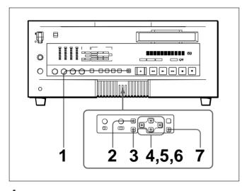
Press the COUNTER SELECT button to light the time data type indicator "TC" or "U-BIT".
